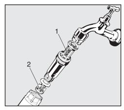
Install the filter (supplied in accessory pack) between the stopcock valve and the inlet hose. The filter for AD water is made of chromium-nickel steel and can be recognised by its dull surface.
